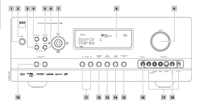
1 POWER BUTTON: Press this button or the HTR 3 remote's [ON] button to switch ON the T 765. The Standby LED indicator will turn from amber to blue and illuminate the VFD. Pressing the power button again turns the unit back to standby mode.
